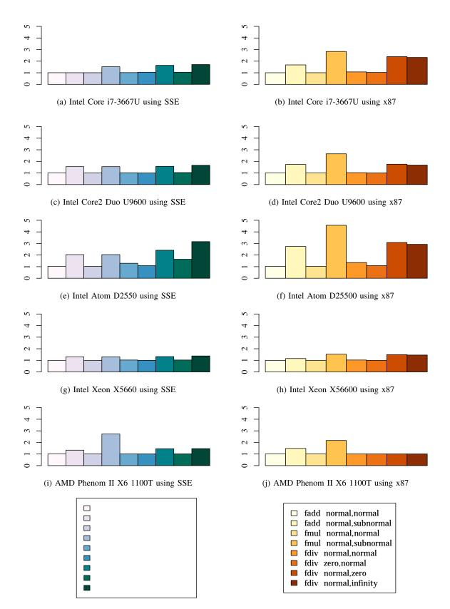
Figure 3: Timing variability of instructions based on input operands. Each test measures the time taken to complete a sequence of loading two values from memory into registers, performing the specified operation using the registers as input, and storing the result back in memory. The y-axis gives the ratio of time taken to perform the specified operation versus the time taken to perform an addition between two normal numbers.
