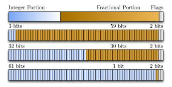
Figure 11: 3 possible internal layouts of a LibFTFP fixed. LibFTFP supports anywhere between 1 and 61 fractional bits, chosen at library compilation time.
